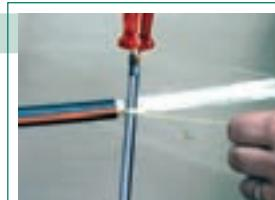
Mount the ripcord with a knot (8 loop) on a screw-driver.
