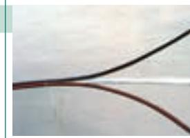
Remove the cable sheath carefully. Cut back the sheath, glass armouring, ripcords and the strength members.
