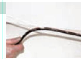
Remove the cable sheath and the strain-bearing elements.
